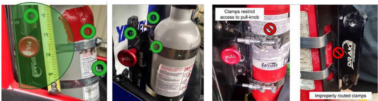
Figure B-54.2: Fire Extinguisher Mounting, Do's and Don'ts
